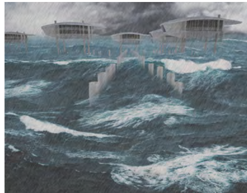
SURGE LANDINGS RAISED ABOVE BASE FLOOD ELEVATION
