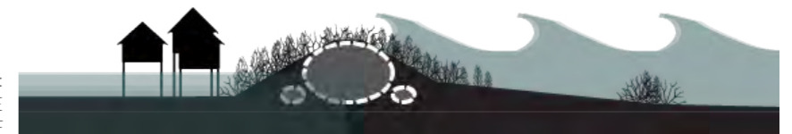
GEOTEXTILE SAND DUNE : SPEED BUMP FOR SURGE APPROACHING FROM GULF
